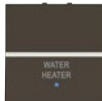
Switch 1-gang, 1-way, DP 20AX, Premium size w/ LED and Heater symbol Rated voltage: 250 Vac Rated current: 20AX Function size: 44 x 44 mm LED indicator and WATER HEATER sign
